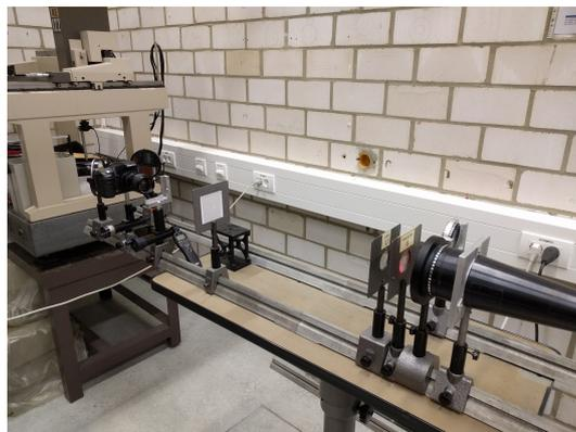
**Figure 6:** Third setup. Note that the lens L1 is directly in front of the grating.
